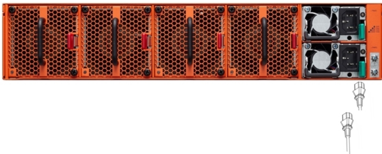
Figure 11 Connecting AC Power on a GigaVUE-TA200
