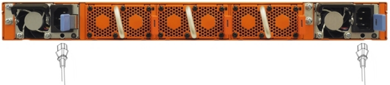
Figure 10 Connecting AC Power on a GigaVUE-TA200
