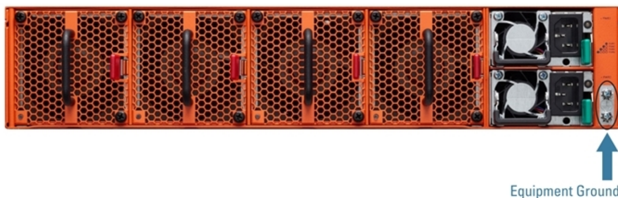
Figure 8 Ground Screws (GigaVUE TA Series-Shown)
